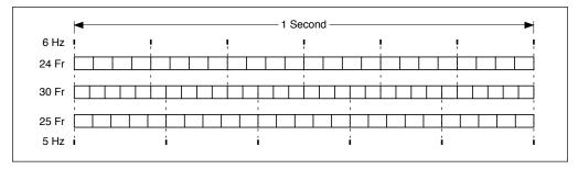
With 24 and 30 f/s, edge coincidence occurs 6 times per second (6 Hz); with 25 and 30, it occurs 5 times per second (5Hz); with 24 and 25, it occurs 1 time per second (1 Hz).
