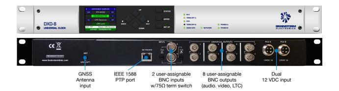
The **DXD-8 Universal Clock** is a precision multi-format reference generator with options for PTP and GPS. It generates 4 independent video syncs and audio clocks simultaneously. With PTP, it acts as a bridge between an IP infrastructure (AES67, ST2110, Dante, Ravenna...) and legacy A/V equipment.
