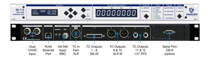
The **SR-112 Time Code Distripalyzer** reshapes and distributes timecode through its 12 outputs, sending it over long lines with no signal degradation. It analyzes the source for quick diagnostic and, with the TCG option, generates or repairs timecode, locked to video if required.
