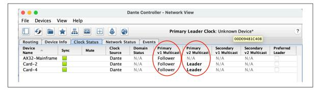
On the other hand, for a cleaner network setup, or if the Dante devices do not have AES67 capability, or to prevent system disruption should a Dante Leader device be taken off-line for any reason, a more robust solution would be to use a second DXD-16 port as a direct master for the non-Dante v2 devices. In the settings below, we will use **port 2**.
