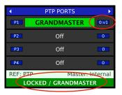
After the successful completion of test 2, you have confirmed that the DXD-16 is recognized as the Best Master Clock.
