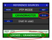
After the successful completion of test 2, you have confirmed that the DXD-8 is recognized as the Best Master Clock.
