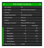
This should be the first thing to check when troubleshooting. Are PTP messages transmitted and received properly by the different devices on the network? If not, some network and switch settings should be checked, especially IGMP and DSCP values and priorities.
